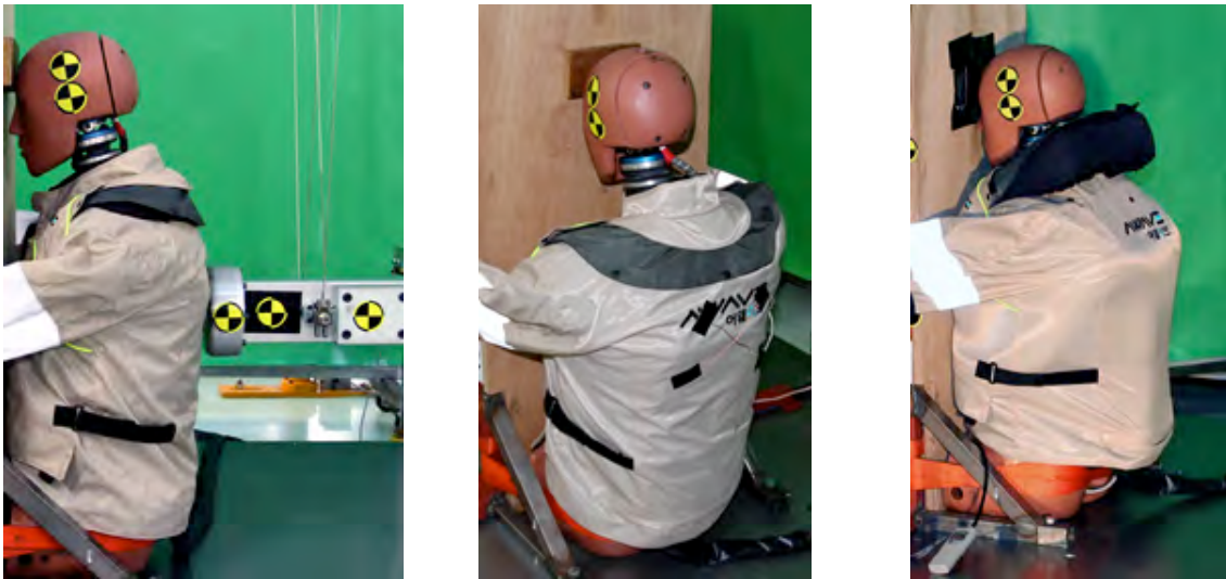
Fig. 1 Jacket clothing conditions in back impact test
