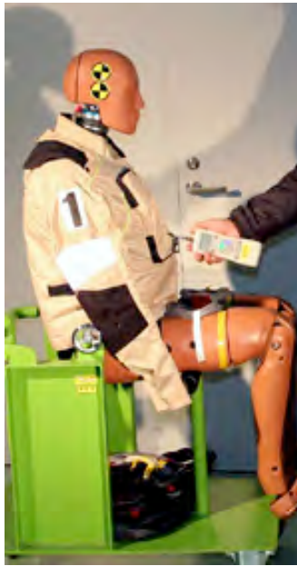
Fig. 4 Jacket inflation time test
